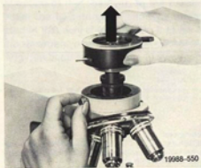
Fig. 22 Removal of the intermediate optical system
