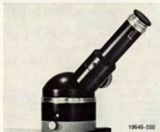
Fig. 3 Inclined monocular pol tube P 12 Standard equipment for monocular observation, fitted with disengageable Bertrand lens. Disengageable pinhole stop for conoscopy of small grains. Application: Wright eyepiece and micro-attachment for the LEICA®.
